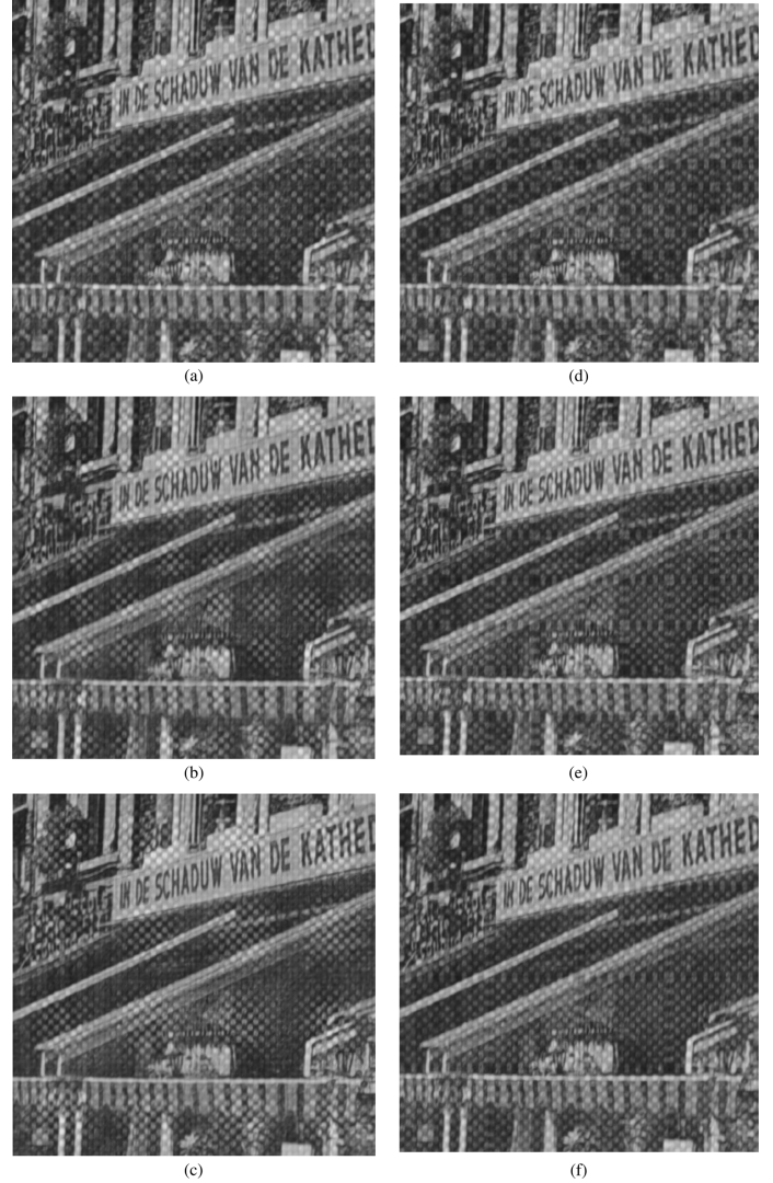
Fig. 6. Part of magnified image with watermarking: (a) 4 \times 4 pixels, DCT, DC = 150, HC = 15; (b) 8 \times 8 pixels, DCT, DC = 150, HC = 15; (c) 16 \times 16 pixels, DCT, DC = 150, HC = 15; (d) 4 \times 4 pixels, WHT and Haar DWT, DC = 150, HC = 15; (e) 8 \times 8 pixels, WHT and Haar DWT, DC = 150, HC = 15; and (f) 16 \times 16 pixels, WHT and Haar DWT, DC = 150, HC = 15.
